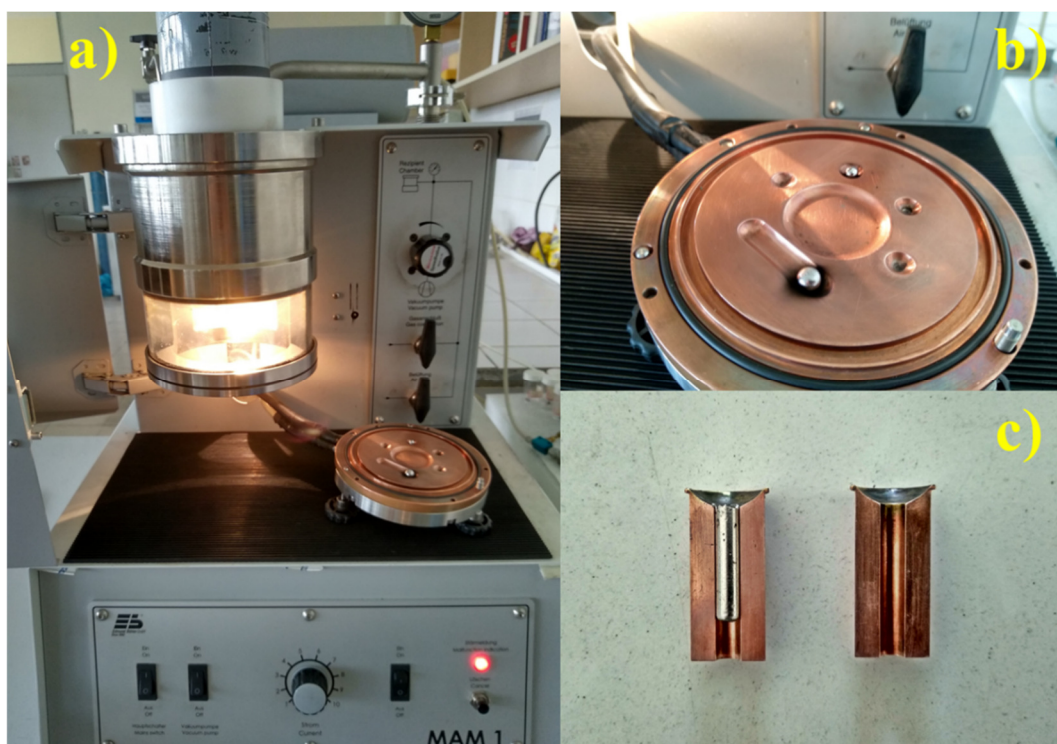
Figure 3.4. Vacuum Arc Melter a, b) Equipment c) Copper suction molds.
